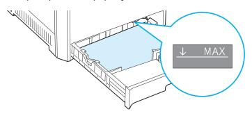
6 Pinch the paper guide, as shown and move it towards the paper until it lightly touches the side of the stack. Do not press the guide too tightly against the edge of the paper as the guide may bend the paper.
